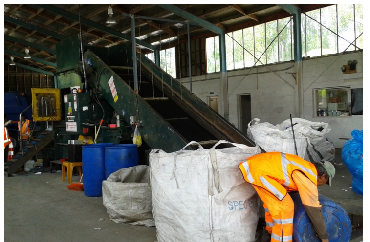
Below: The Baler installed and working at Croad Place.
